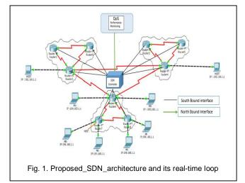
In our developed architecture, there are three cloud interfaces 4 Comparison Between The Internal And with nine switches. These numerous switches are associated with eight hosts which have possessed IP address. For observing QoS exhibitions from hosts to switches, SDN controllers are utilized like existing controllers and outer controllers.
